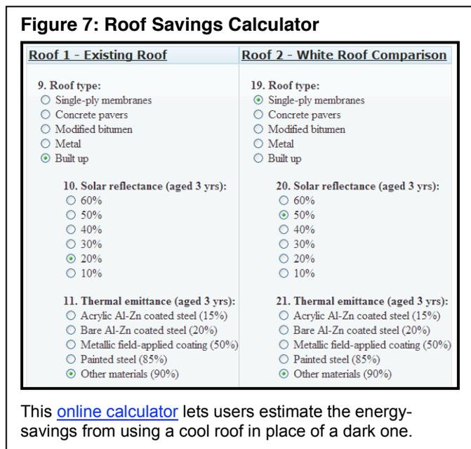
*Climate* has the biggest impact on energy savings. Cool roofs achieve the greatest cooling savings in hot climates (Climate Zones 1-3; see Figure 8) but can increase energy costs in colder climates due to reduced beneficial winter time heat gains. The DOE Cool Roof Calculator takes into account your local climate when you select the state and a city nearest your building.
